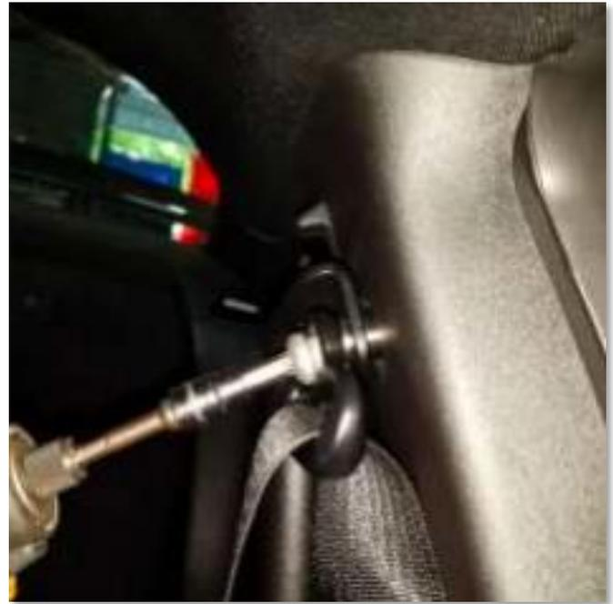
*Figure A.6 – Removing a shoulder point bolt*
