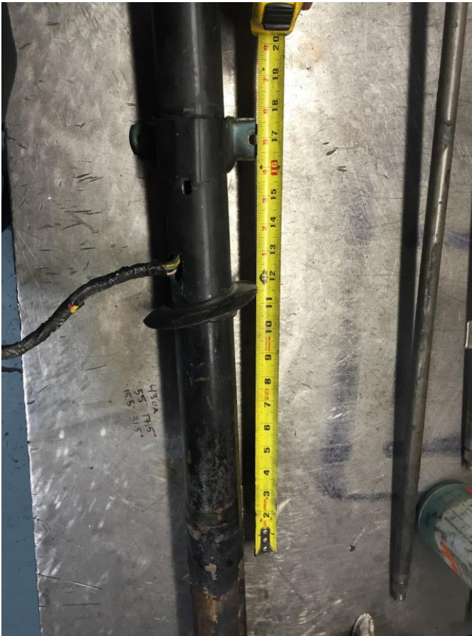
D.4 – With the bracket placed on the steering column in the original location, the measurement from the previous step can be used to draw your cut line.
