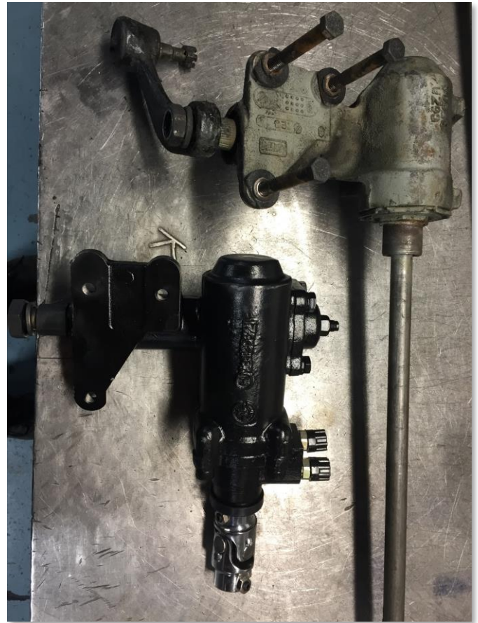
Figure B.7.3 – A side-by-side view of the original factory box and the new power steering box.
