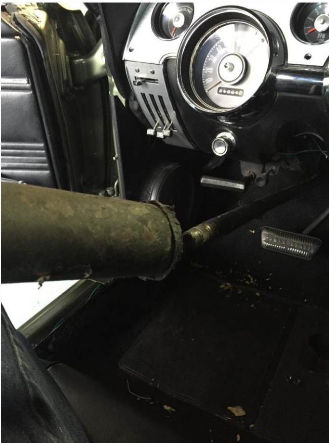
Figure B.4.2 – The steering column can now slide off the steering shaft.
