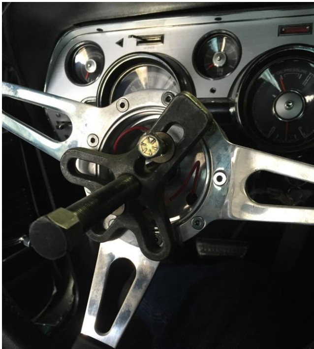
Figure B.2.1 – Steering wheel puller being used to remove steering wheel
