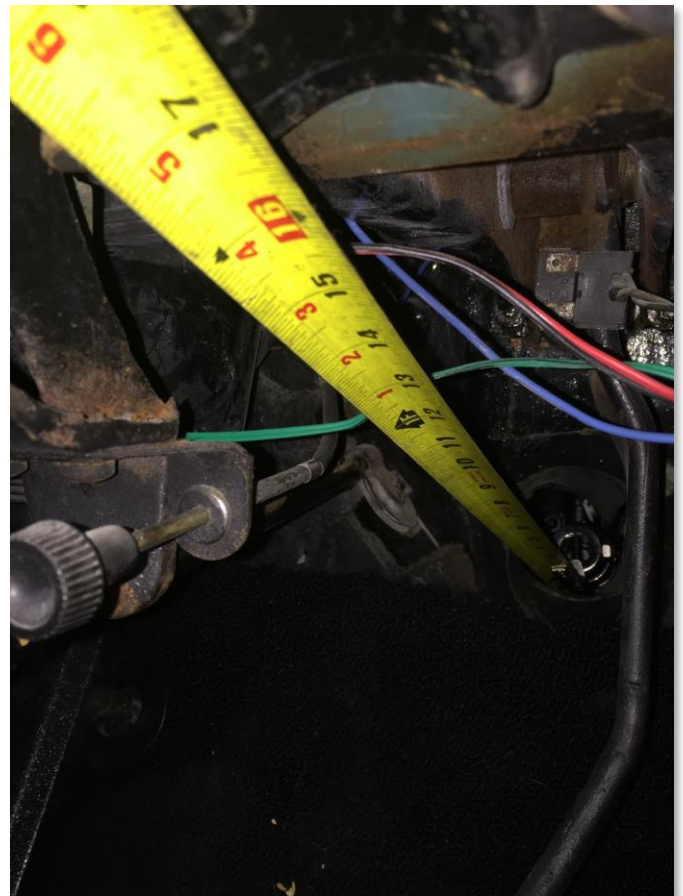
Figure D.2 – Measuring the distance from the steering column bracket to the center of the universal joint.
