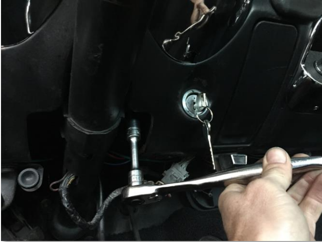
Figure B.4.1 – Removing the u-shaped bracket used to secure the steering column to the dash.
