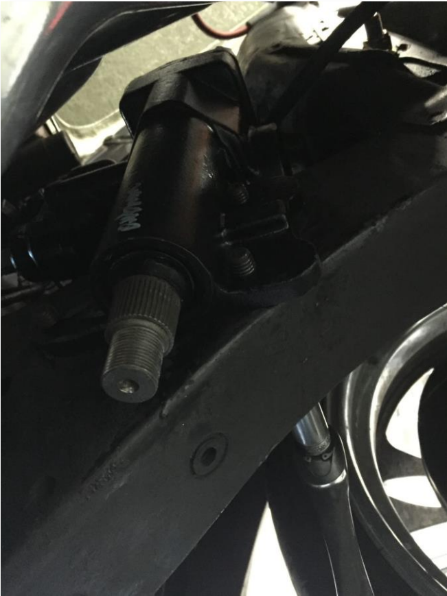
Figure C.2 - Installing the new power steering box
