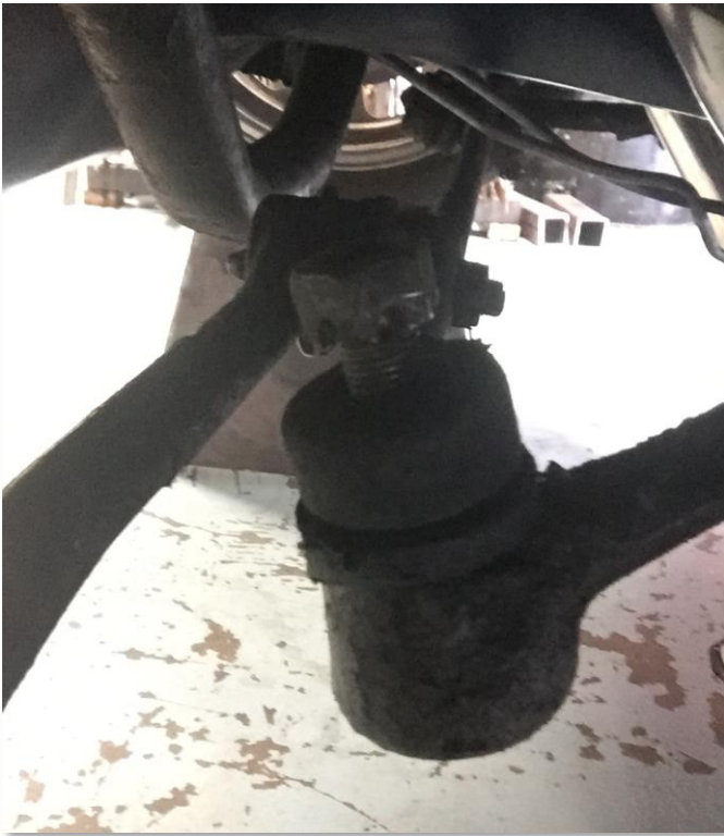
Figure B.6.1 – The castle nut installed upside-down to protect the threads
