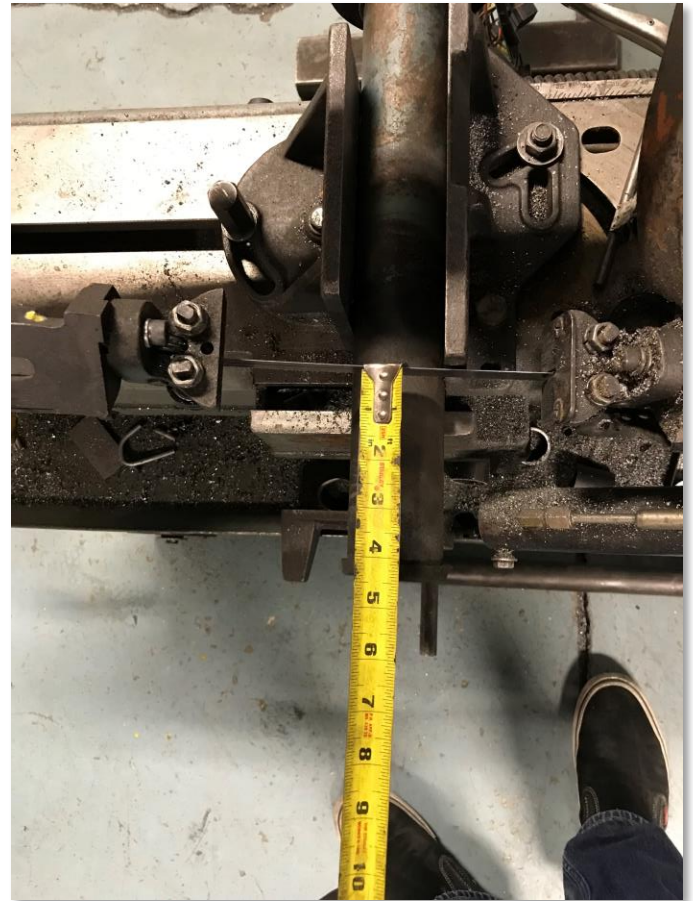
Figure D.5 – Here is the column clamped up in the bandsaw ready to be cut.
