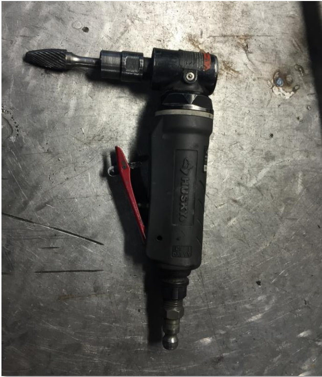
Figure C.1 – We used a die grinder to open up the lead lower hole
