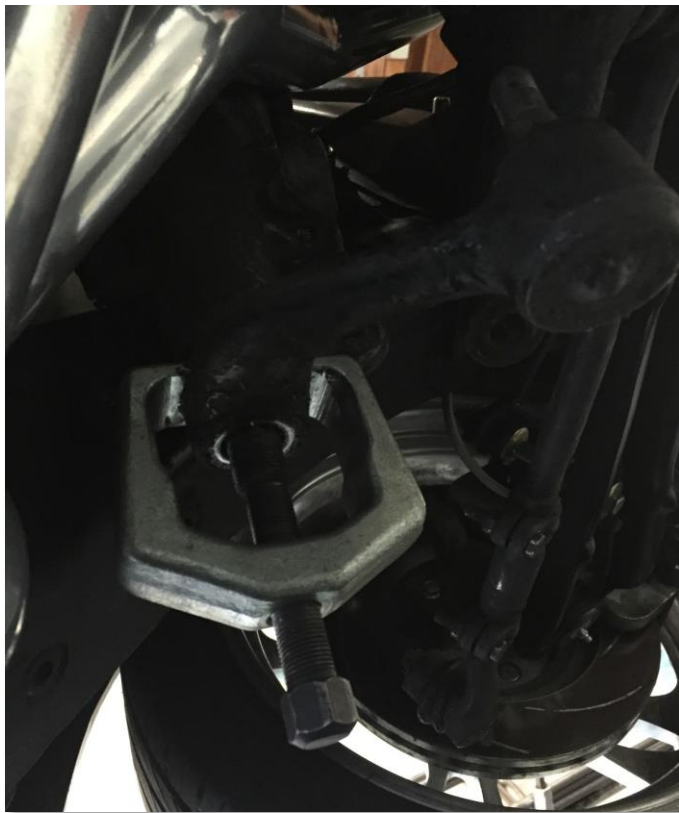
Figure B.6.2 – Here a pitman arm puller is used to separate the pitman arm from the steering box.
