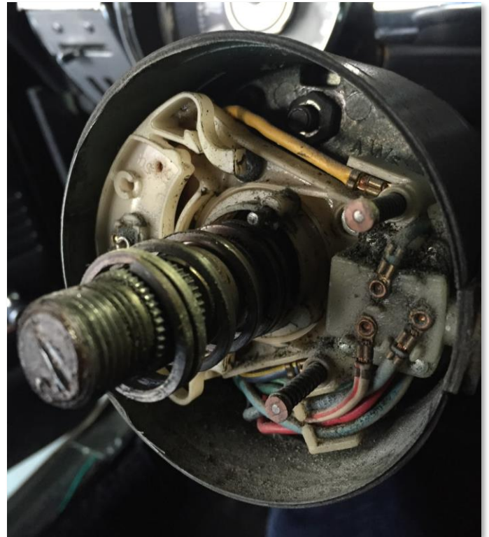
Figure B.2.2 – The steering wheel has been removed, be sure not to lose any of the hardware
