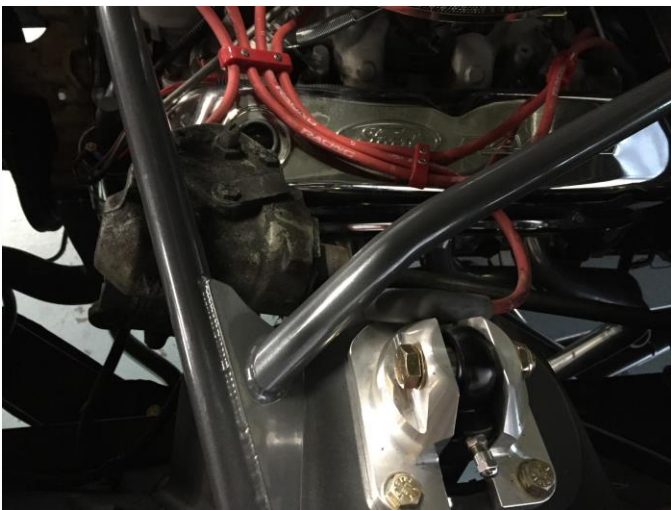
Figure B.7.2 – A view of the steering box being removed from a 64-66 Mustang, notice how it is removed by sliding it forward over the headers.
