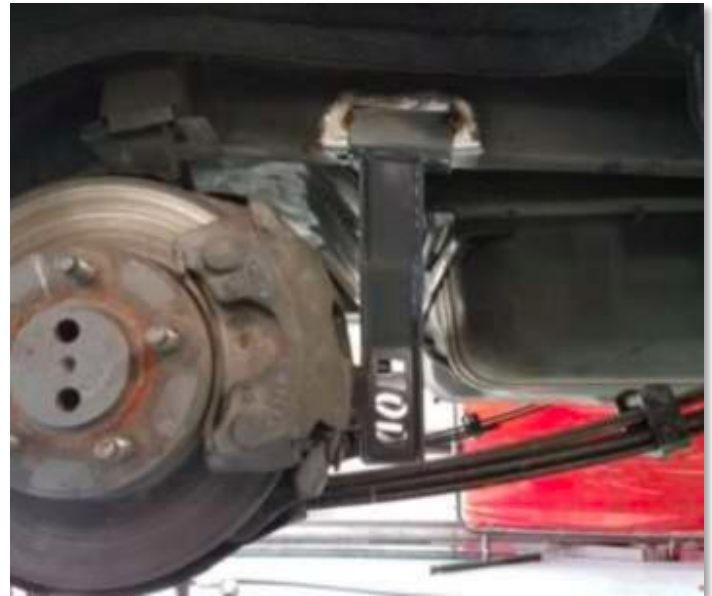
B.3 - Panhard bar chassis bracket tack welded in 2 locations
