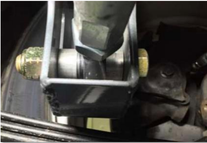
E.4 - Chassis bracket with panhard bar bolted in
