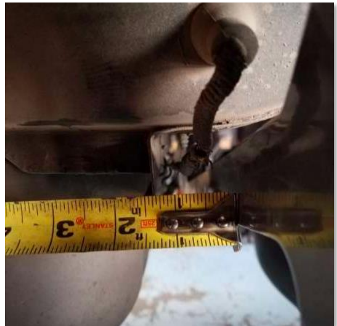
A.6 - Referenced measurement for alignment to front flange of fuel tank. Measurement shows approximately 1 3/8" whereas 1 1/2" is desired.
