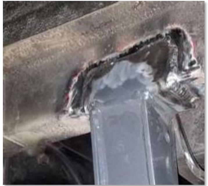
D.2 – Driver's side of bracket, stitch welded to the frame rail
