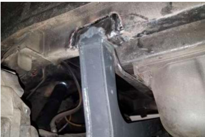
Drivers side view showing clearance for exhaust and fuel system.
