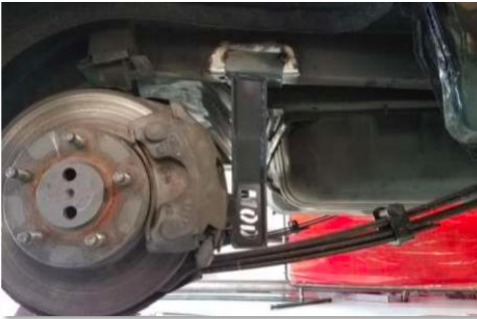
On vehicle fitment for clearance of exhaust, fuel lines
