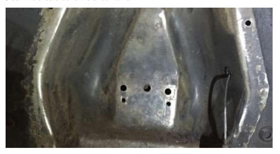
Figure 6 Shock tower wire wheeled and pilot holes drilled for Shelby drop on a 1964.5-1966 Mustang
