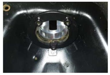
Figure 9 Shock top assembly installed
