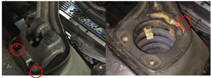
Figure 2 Shock & Shock Cap Removal.
