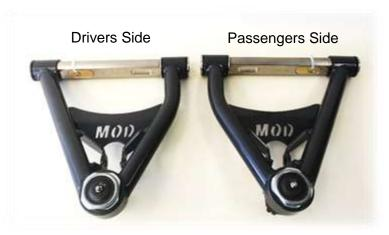
Figure 1. Notice the orientation of the control arms. The arrow in the shaft assembly should be pointing towards the front bumper and the bent leg of the control arm should be on the rearward side of the vehicle. The yellow zinc plated alignment key may need to be flipped from factory installation depending on application.
