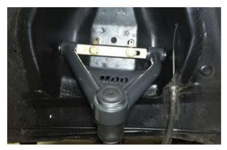
Figure 10 Upper control arm installed in vehicle. Note: Front of vehicle is on left side of the page
