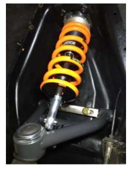
Figure 11 Coilover shock partially installed.
