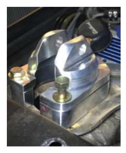
Figure 7 Shock top & spacer fitted to confirm the need to modify.
