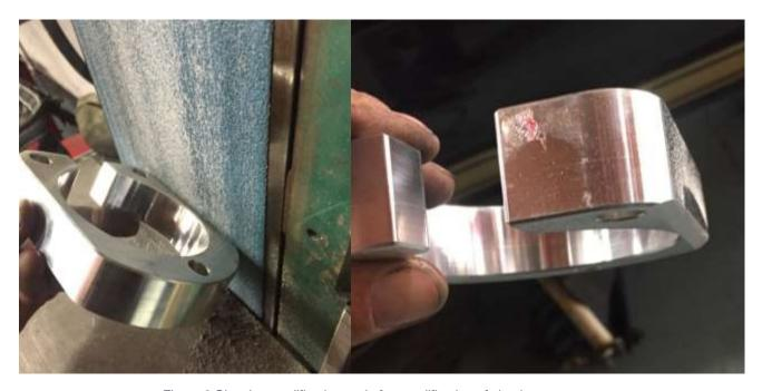
Figure 8 Showing modification and after modification of shock spacer.
