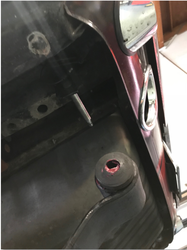
Figure D.2 – Here the leaf spring is about to be lifted onto the shackle assembly. Note the orientation of the shackle bolts.
