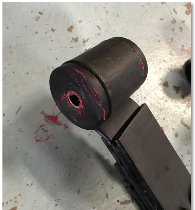
Figure D.1.3 – A view of the completed installation of the front eyelet bushings.
