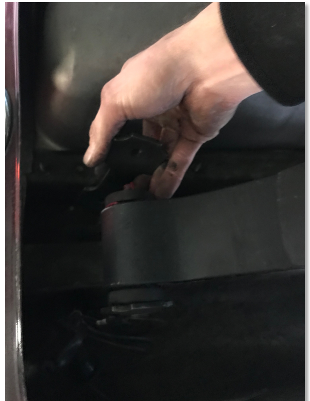
Figure D.5 – Here the remaining shackle plates are being installed.
