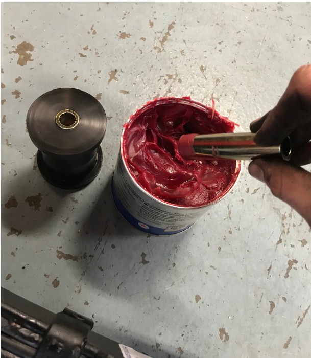
Figure D.1.1 – Applying grease to eyelet bushings and collar
