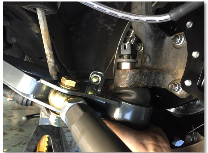
Figure D.2.2 Install the castle nut, and torque to spec
