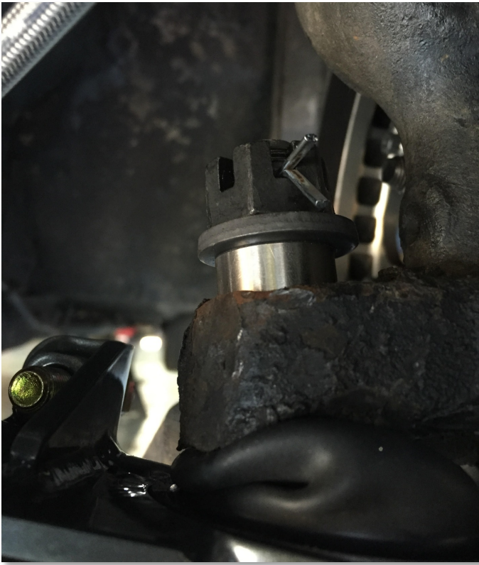
Figure D.2.3 – Complete this step by installing a new cotter pin.
