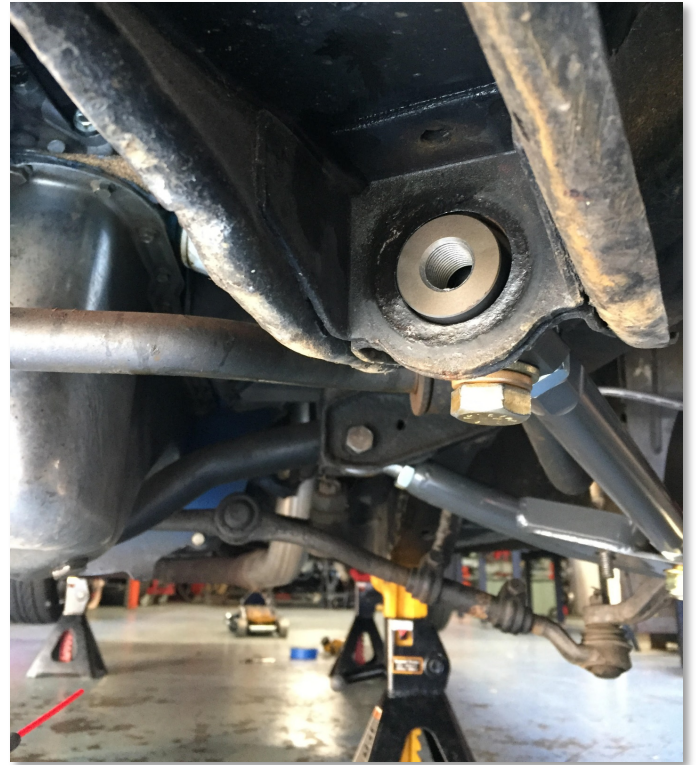
Figure E.1 – A view of the strut rod fitted to the mounting point on the chassis.
