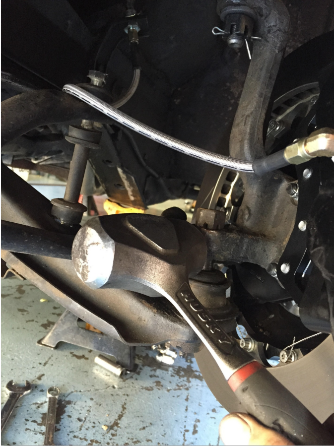
Figure C.3 – We have just knocked the bolt loose from the spindle. You can see the lower control arm has dropped free. The installed castle nut also prevents it from falling on the floor.
