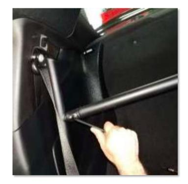
Figure C.1 – Bolting the harness bar to vertical members
