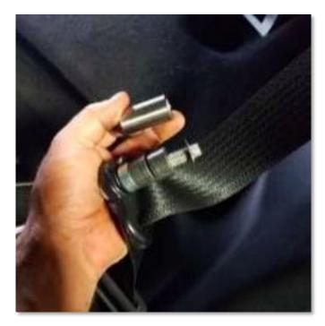
Figure A.7 – Showing the disassembly of the stock spacers
