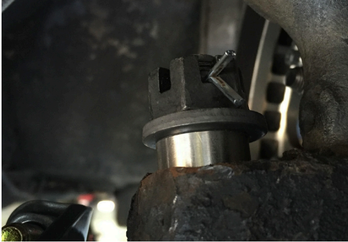
Fig. 13 - Complete this step by installing a new cotter pin.
