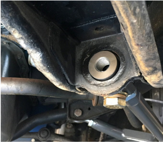
Fig. 14 - A view of the strut rod fitted to the mounting point on the chassis.
