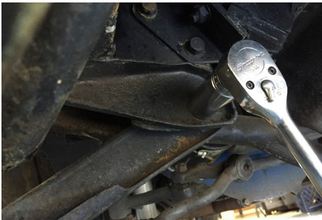
Fig. 4 - Unbolting the control arm from the chassis.
