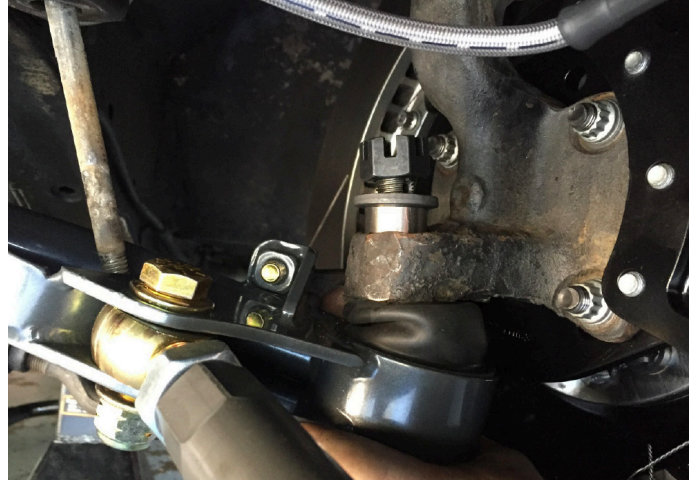
Fig. 12 - Install the castle nut and torque to spec (60-90ft-lbs)
