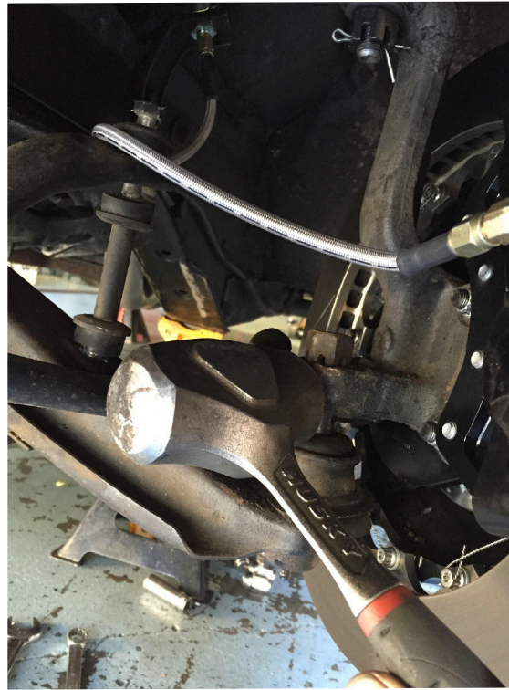
Fig. 6 - We have knocked the bolt loose from the spindle. The lower control arm has dropped free.
