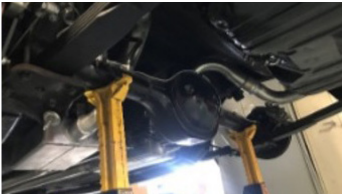
Fig. 1 - Jacks support under rear end housing.
