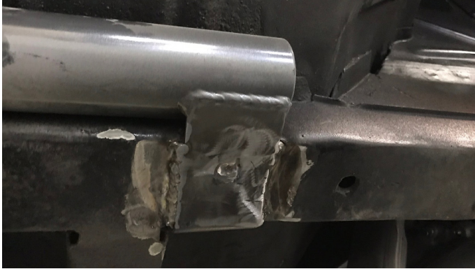
Fig. 16 - Bracket #1 Front bracket welded.
