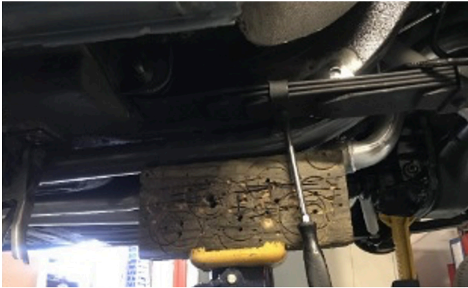
Fig. 12 - Check clearance of leaf spring.
