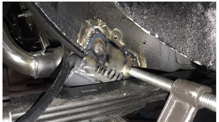
Fig. 19 - Bracket #4 Rear frame rail box welded.
