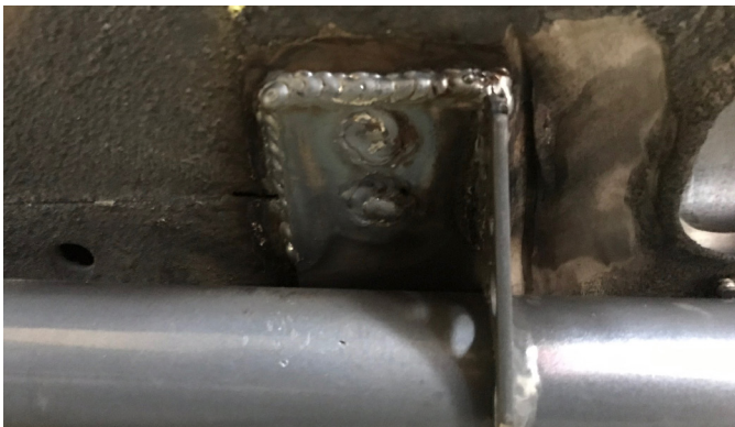
Fig. 18 - Bracket #3 Torque box bracket welded.
