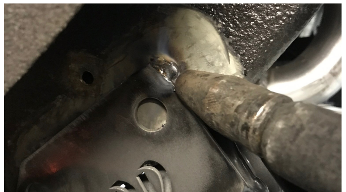
Fig. 15 - Tack weld final bracket.
