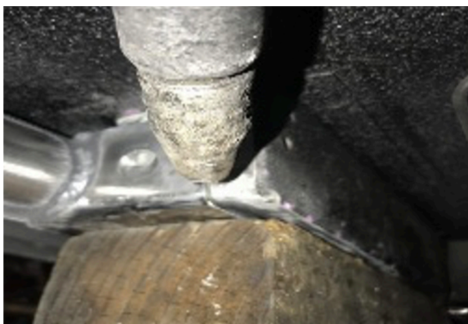
Fig. 10 - Use block of wood on jack to push up on brackets.
