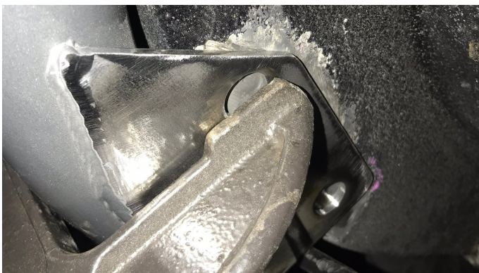
Fig. 14 - Use a clamp to keep bracket #4 snug against frame rail during tack welding.
