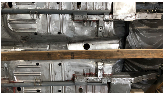
Fig. 8 - Connector lined up and fit into place.
