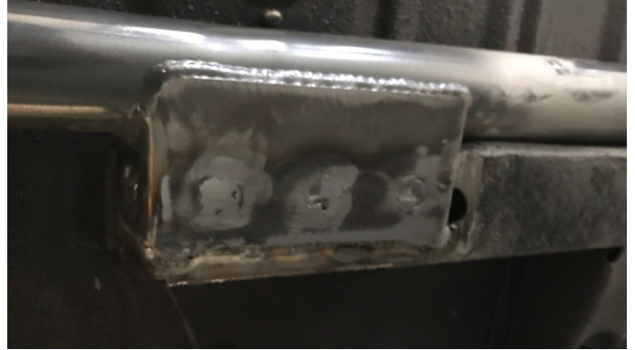
Fig. 17 - Bracket #2 Pocket bracket welded.
