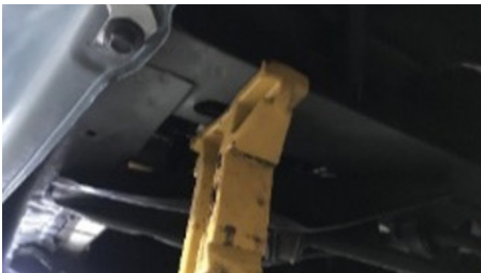
Fig. 3 - And jack under the front of cross member.
