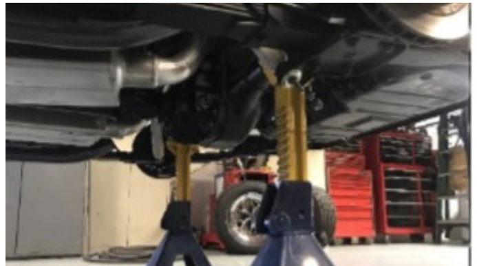
Fig. 2 - Jack under rear end housing.
