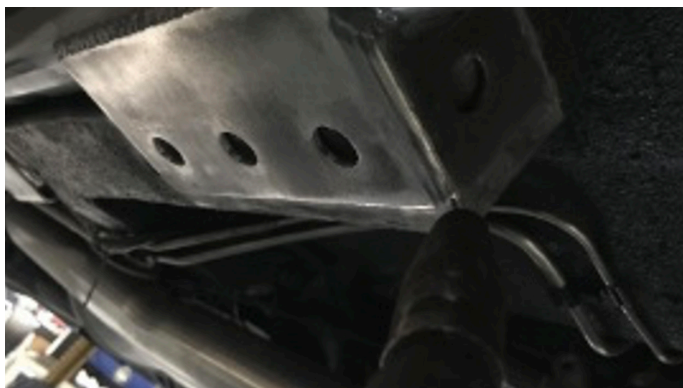
Fig. 9 - Start with a tack weld on bracket #2.
